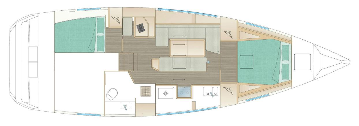
2 cabin version: 1 aft cabin on portside, 1 convertible aft locker on starboard, 1 large heads, 1 fore owner cabin & 1 fore locker
