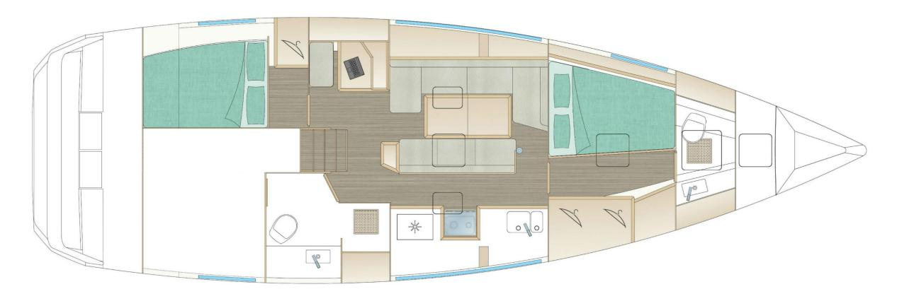
2 cabin version: 1 aft cabin on portside, 1 convertible aft locker on starboard, 1 large heads, 1 fore cabin on portside, 1 fore heads & 1 fore locker
