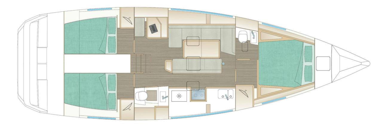
**3 cabin version**: 2 aft cabins, 1 heads on starboard, 1 fore owner cabin, 1 heads on portside & 1 fore locker
