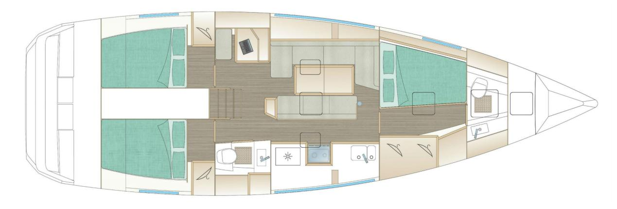
3 cabin version: 2 aft cabins, 1 heads on starboard, 1 fore cabin on portside, 1 fore heads & 1 fore locker
