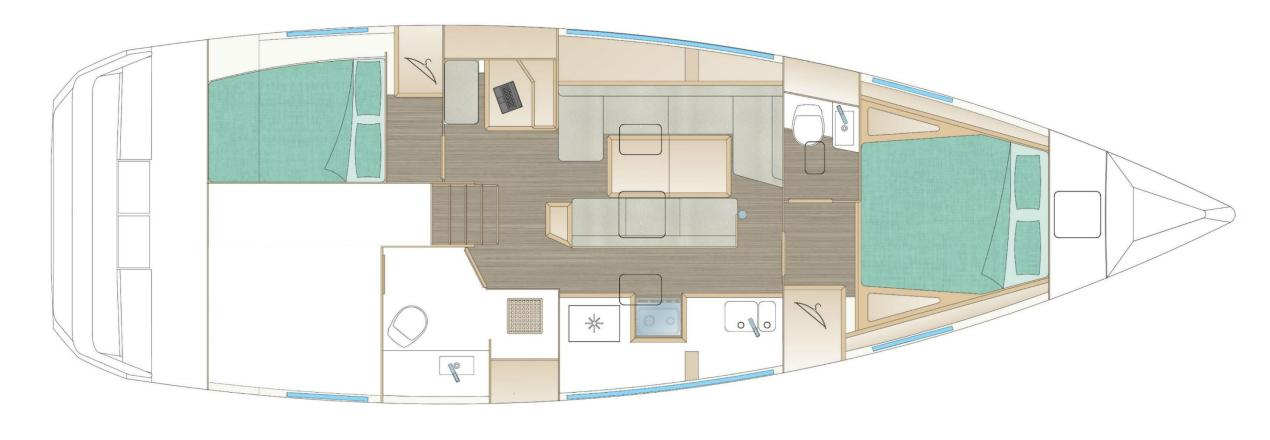
2 cabin version: 1 aft cabin on portside, 1 convertible aft locker on starboard, 1 large heads, 1 fore owner cabin, 1 heads on portside & 1 fore locker
